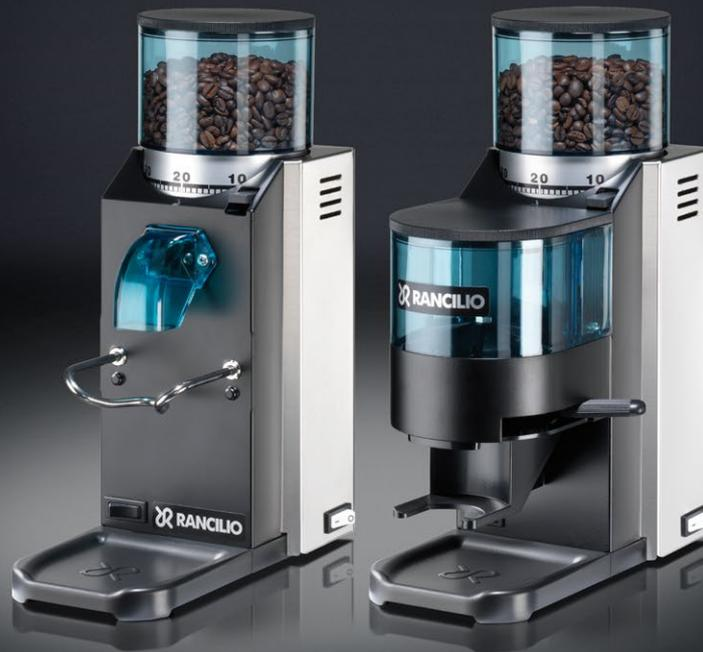
**Rocky** has grinding burrs with a diameter of 1.9 inch (50 mm), guaranteeing a production of 5.5-7.7 lb/hour (2.5-3.5 kg/h). The dosage is 0.2 oz (7 g), with a capacity for 10.5 oz (300 g) of coffee beans. Semi-automatic version.
